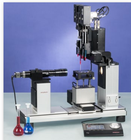
determination of the surface energy using an OCA 200 with DDE/4 and four ESr-N
